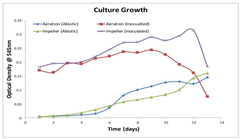
Inoculated chamber with impeller pump showed higher overall growth - All four chambers reached peak growth around day 10
