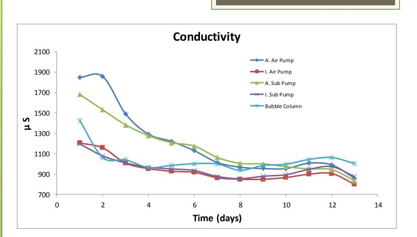
Conductivity reduces with time because of ammonia volatilization as well as uptake of other ionic nutrients. (i.e. K<sup>+</sup>, Mg<sup>2+</sup>)
