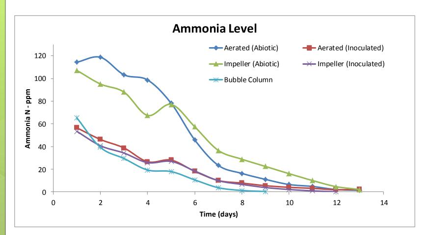
All systems reduced ammonia levels below Groundwater Cleanup Target Levels of 2.8 ppm (FL DEP) in 12 days
